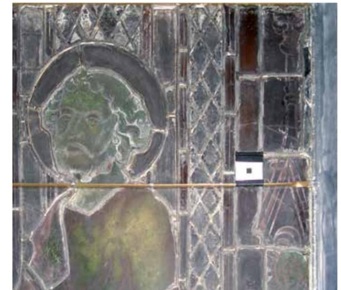
Fig. 1 - Glass sensor on the inside
